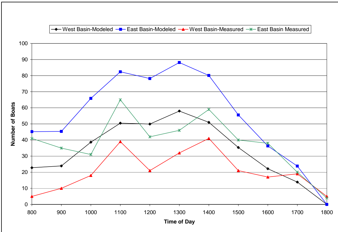
Figure 3-5 – Measured vs. Modeled Outbound Traffic
